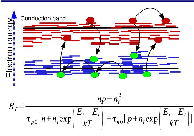
This is often done using the following **SRH** equation, which assumes a *steady* state distribution of trapped charge carries in the trap states.
